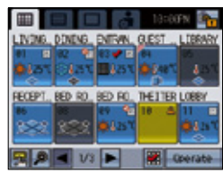
GRID (zoom-in) screen Displays the detailed operation status of each group.
